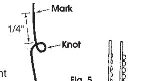
Reinstall cord on top guide of Laserguard. If too tight reposition the knot on cord. Once this operation is complete, you can cut off excess cord.
