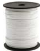
H 6038 #3 1/2, 7/64" Nylon braid, Fiberglass core Traverse Cord 100 Yard Roll
